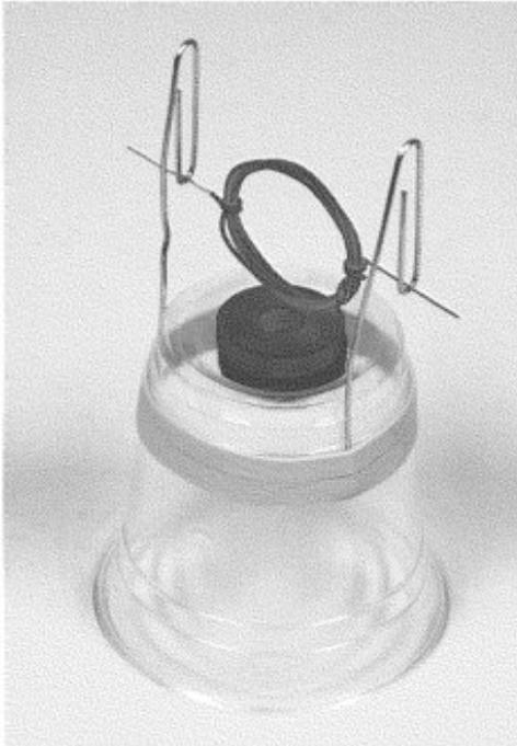
10. Adjust the coil and the clips until the coil stays balanced and centered while spinning freely on the clips. Good balance is important in getting the motor to operate well.
