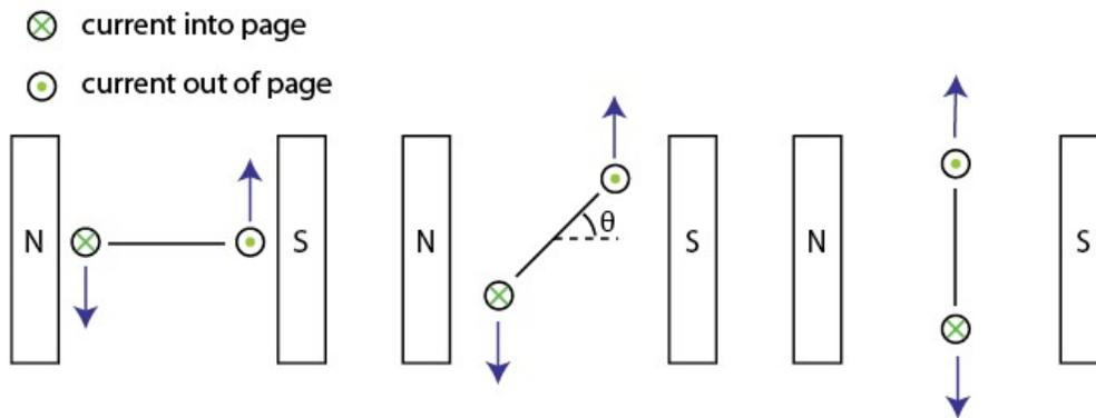
Figure 3: Schematic diagram showing the difficulty with a coil in a magnetic field.
