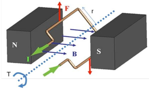
Figure 2: Schematic diagram of a coil of wire conduction current in a magnetic field.
