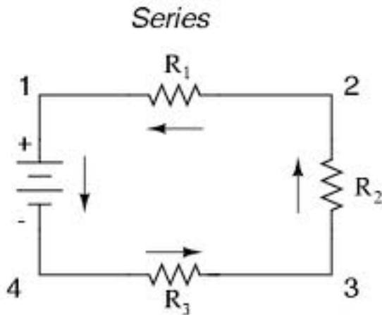
They should describe that the electrons are pushed by two batteries through a wire that passes through resistor 3 then a wire to resistor 2 then a wire through resistor 1 and finally back to the positive terminal of the battery. This is an example of a series circuit.
