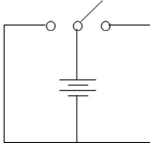
Buttons perform a very similar operation but when the button is not pressed the circuit goes back to its original path. For example, if the button were set to its normal position, the current would flow that way continually until the button was pushed to change the direction of the circuit. How would the circuit above change if there was a button instead of a switch? Have your students brainstorm the pros and cons of using a button instead of a switch.
